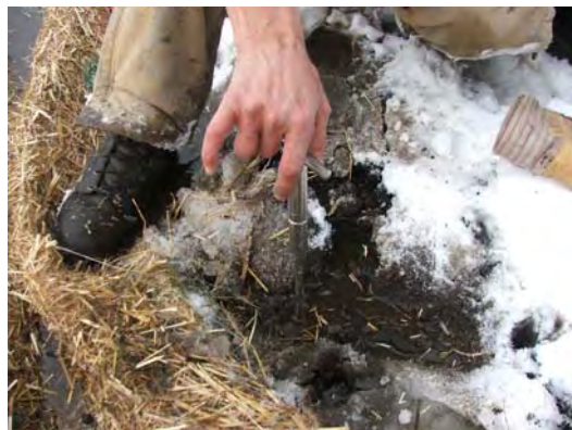
Envirocon batch plant shuts down due to clogging. Soil shear strength testing along northern alignment.
