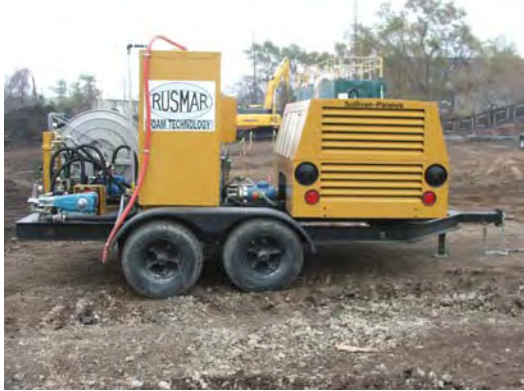
Odor controlling foam machine arrives.
