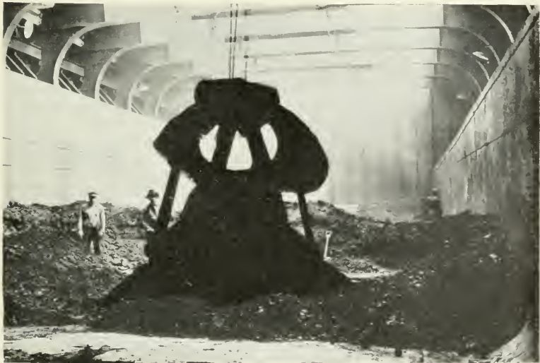
PLATE 6.—A 5-ton Clam Shell in the hold of a Lake Freighter. The picture indicates the construction of the boats to facilitate rapid, unimpeded unloading.
