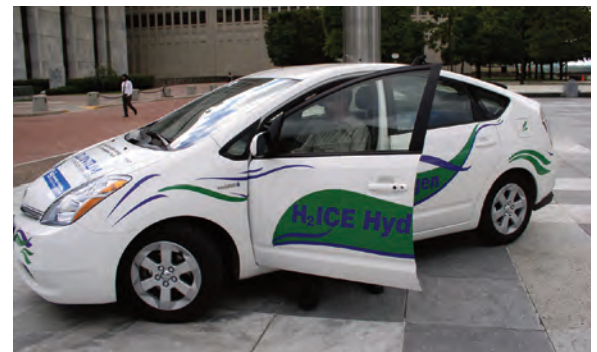
At SUNY-Buffalo, facilities staff are conducting a two-year cold-climate test of a hydrogen-fueled Prius hybrid car, funded by NYSERDA (New York State Energy Research and Development Authority).
