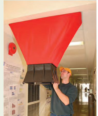
Checking air flow in HVAC system. "Continuous commissioning" is one of Penn State's strategies to maximize building energy efficiency.
