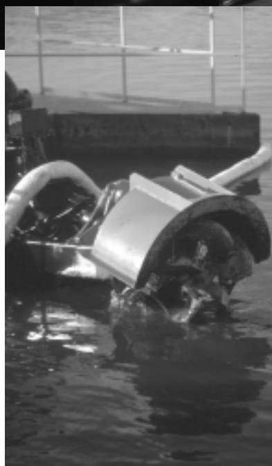
Shielded cutterhead of hydraulic dredge
