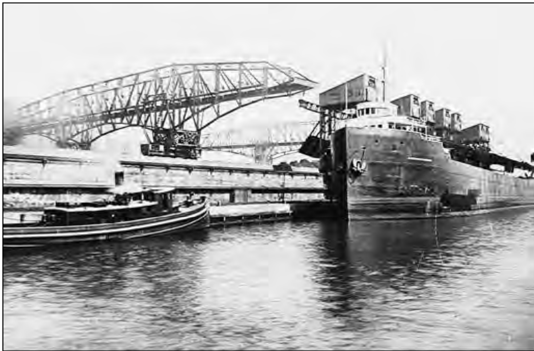
26. Ore boat unloading – The site for South Works was chosen because of its proximity to water transportation. This was most economical way to bring the materials used in the steel making process. Iron ore, limestone, and coal were transported to South Works in huge ore carriers which unloaded their cargoes at slips served by huge overhead cranes. This is a photo of a ship unloading its cargo at the North Slip which connected to Lake Michigan.
