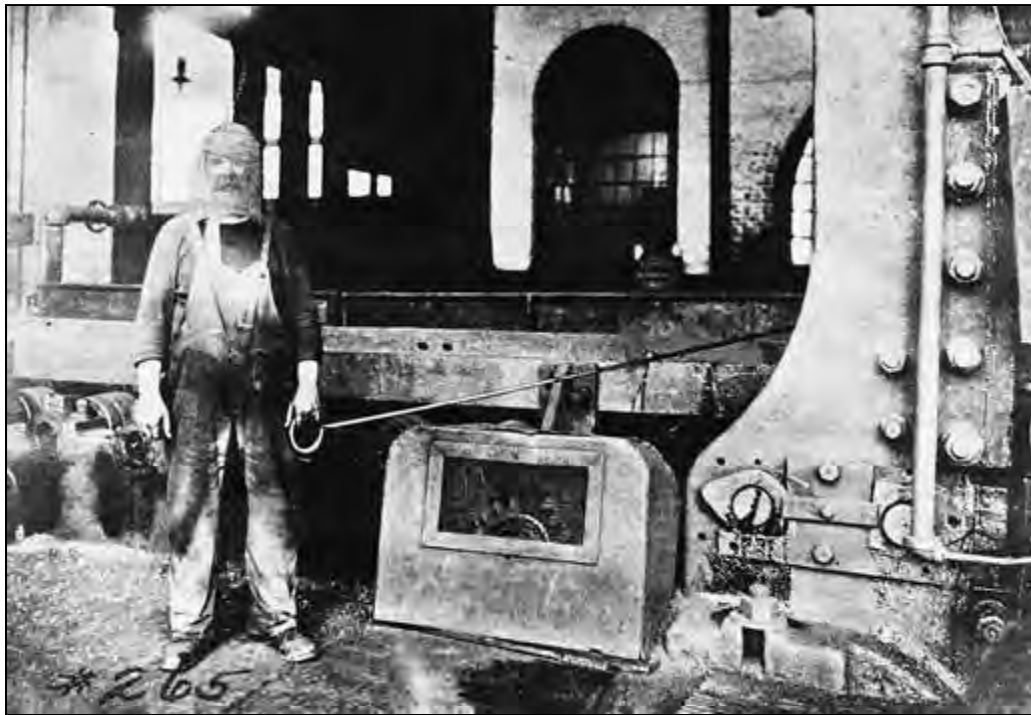
29. Early safety mask – In 1905 Robert J. Young began a study of injuries at South Works. In 1906 the South Works Safety Committee recommended 3,000 changes in plant operations. In 1908 U. S. Steel began a safety program based on the South Works model for the entire corporation. This early, primitive net safety mask from 1890 provided some protection for a worker.
