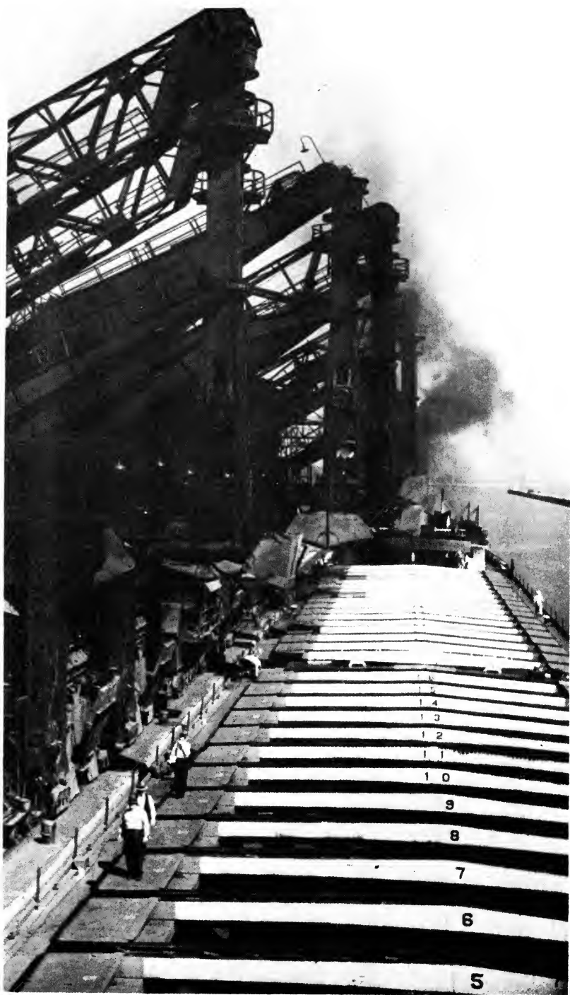
"12,000 Tons of Ore Have Been Unloaded in Less Than Four Hours by Seven Electric Ore Unloaders" — Gary Harbor
