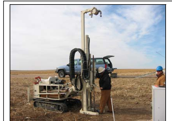
Soil sampling using a geoprobe. Source: http://www.usgs.gov/
