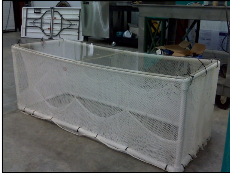
Figure 1 – 3. Protective netting, frame, and cover for the exposure tank. A frame constructed from PVC pipe was covered with a double layer of cloth netting and inserted into the exposure tank to prevent silver carp from making contact with the sides of the tank and electrodes. A clear Plexiglass cover prevented silver carp from leaping from the exposure tank during the electrical treatments, while allowing visual observation of fish responses. The pilot study was conducted at the USACE, ERDC-EL, Vicksburg, Mississippi 20-24 April 2009.
