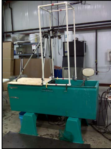
Figure 2 – 3. Exposure tank for the experiments in the screening trial. Experiments in the screening trial were conducted in a 168 cm x 42 cm rectangular fiberglass tank (water depth was 40 cm). Plate electrodes were used to create a homogeneous electric field in the tank. Each simulation was video recorded. The screening experiments were part of a more comprehensive study of operational protocols for the electric barriers on the CSSC, conducted at the USACE, EL-ERDC, Vicksburg, MS, 3 September to 30 December 2009.
