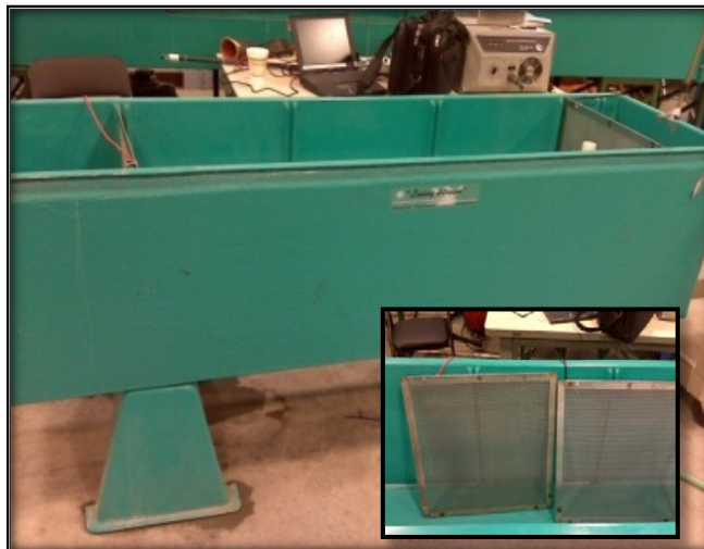
Figure 1 – 2. Exposure tank. Small silver carp were exposed to electrical treatments in a 530 liter (l) dielectric tank in the pilot study on operational protocols for electric barriers on the Chicago Sanitary and Ship Canal. Flat, perforated, stainless steel electrodes (insert) were positioned parallel to one another in the tank, covered the entire cross-section of the tank, and extended above the surface of the water, creating a homogeneous electric field. The experiment was conducted at the USACE, ERDC-EL, Vicksburg, Mississippi 20-24 April 2009.
