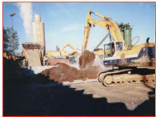
Mixing dredged material and treated contaminated soil to create aggregate for construction materials in New York. Credit: New York State Dept. of Environmental Conservation.
