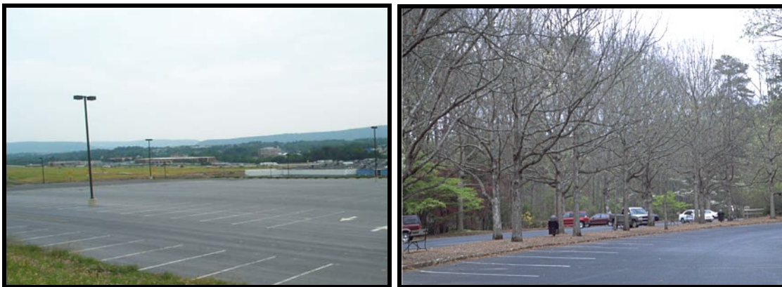
Figure 40. Parking lot with no landscaping (left) and a double-wide interior planting strip that allows trees to share rooting space (right, photo by Ed Gilman)
