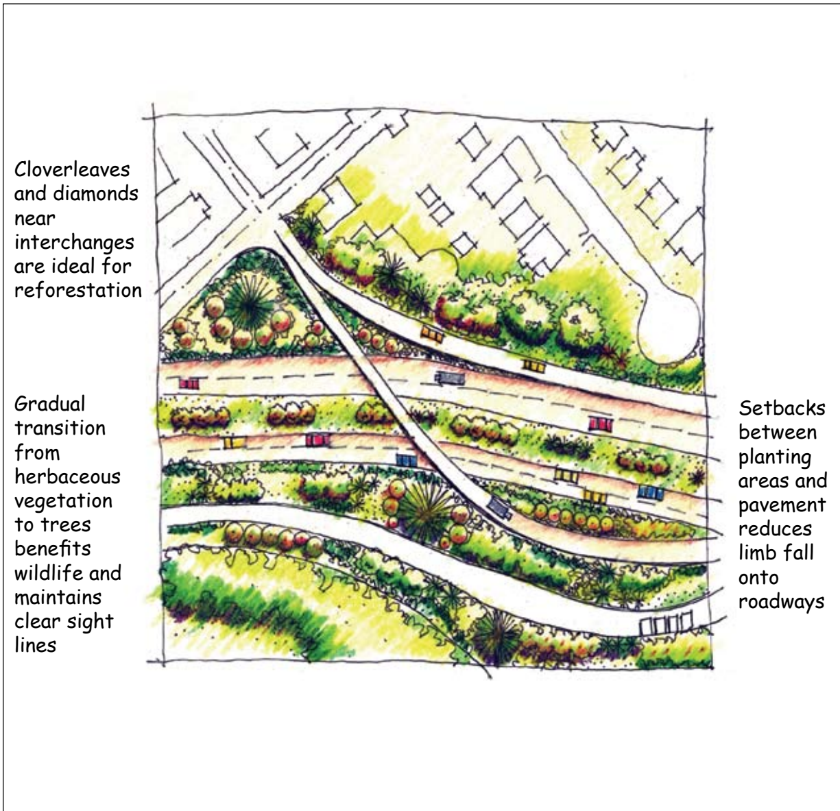
Figure 26. Planting trees in highway rights-of-way
