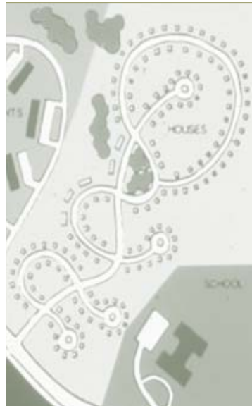
Example of a development plan with cul de sacs which provides limited connections to outside. (source: internet)
