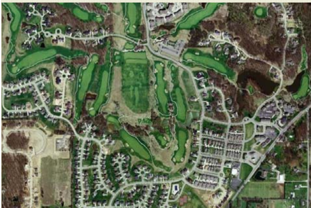
Aberdeen, Valparaiso-IN: A golf course community developed by using PUD zoning. It includes mixed uses, commercial, offices and residential development. The subdivision was planned to preserve natural features.
