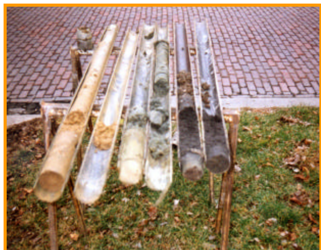
Soil borings are ready for field screening and sample collection.
