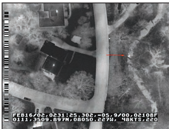
Figure 72: Aerial thermography showing sewage leak
