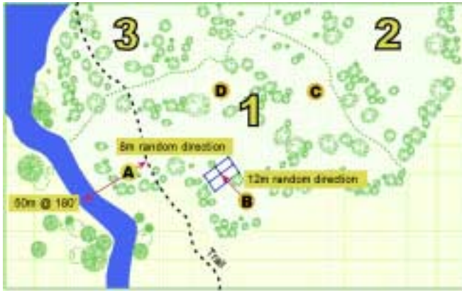
Figure 16. Initial steps of plot location.
