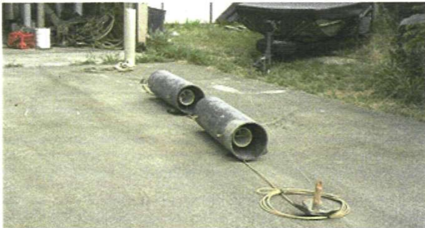
Figure 16. Double shrouded, duplicate in-line rigging used at SEPA Station 5 intake
