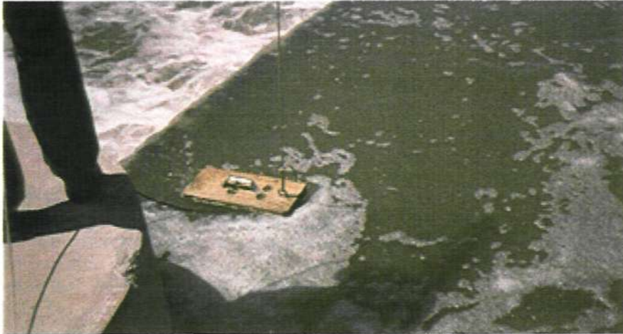
Figure 15. YSI stirrer - DO/temperature probe flotation board used during manual measurements
