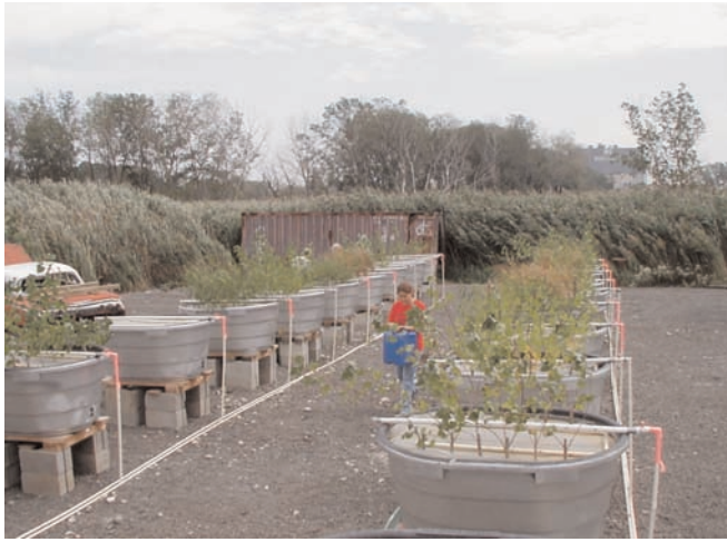
Figure 17.— The trees in this phytoremediation tank experiment grow better in the dirty water because one of the main contaminants is ammonia which acts as a fertilizer. This is part of why phytoremediation works.
