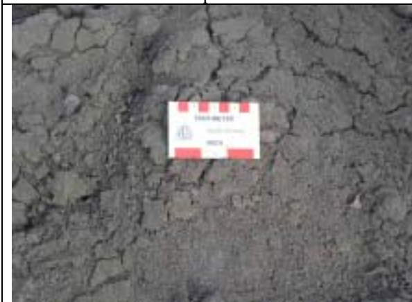
Fig. 25. Sediment at the Powers site showed evidence of soil formation on January 13. The top layer was granular and easily broken apart by hand.
