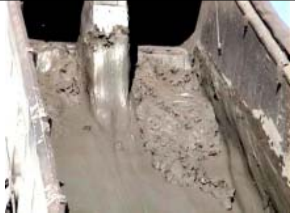
Fig. 18. Small amounts of sediment occasionally hung up in the corners of truck beds. This sometimes was associated with residue from a prior load of another material such as lime.
