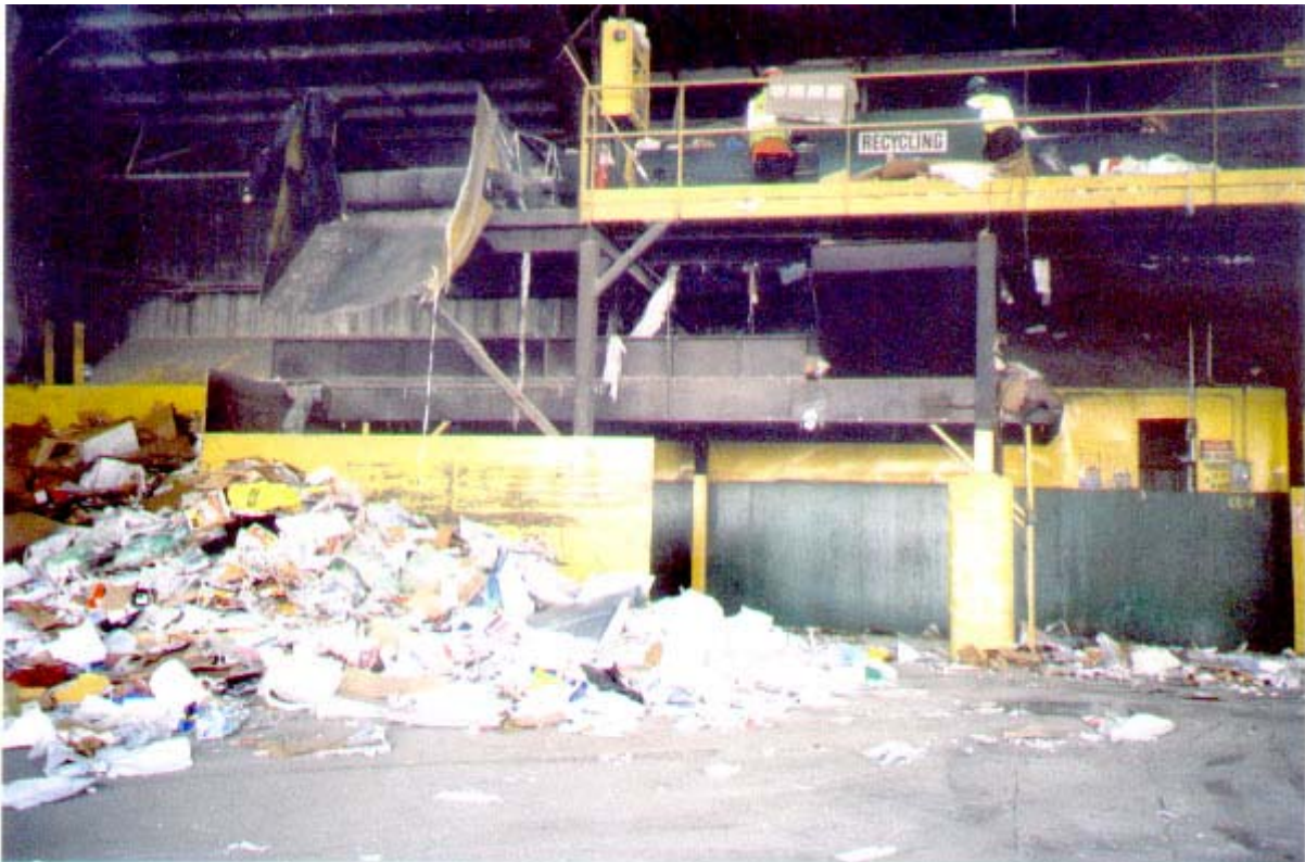
Workers sorting out recyclables from the waste stream at Hooker Street Transfer Station in Chicago. Transfer stations in Chicago are open 24 hours.
