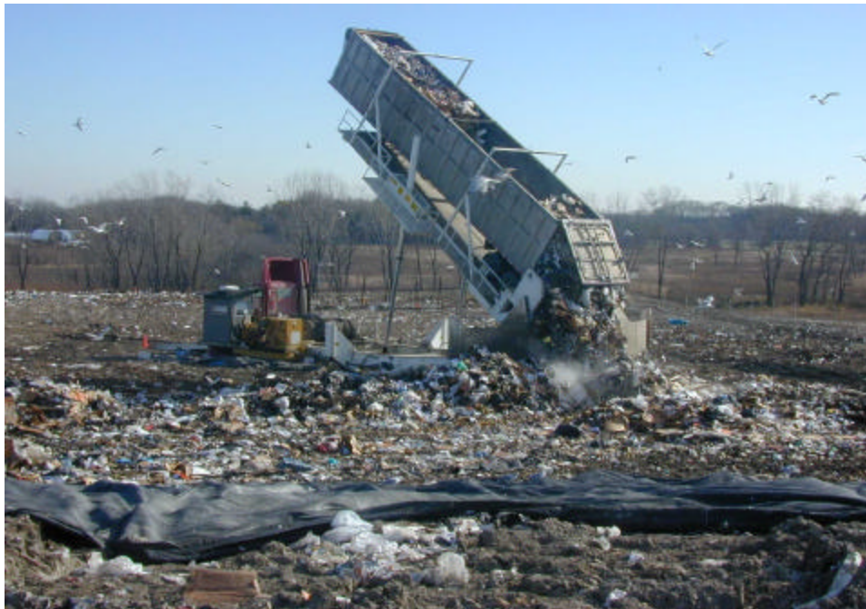
Tipper in active working face at BFI Zion Landfill Site 2, which ranks seventh in Illinois in terms of waste disposed
